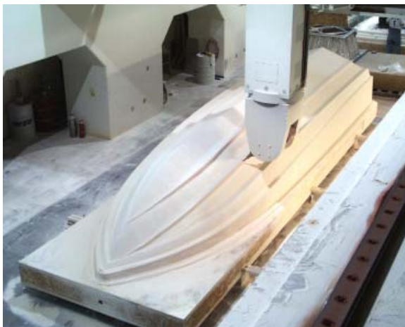
Hull plug machined with Janicki's 5-axis milling machine from Rhino files.
