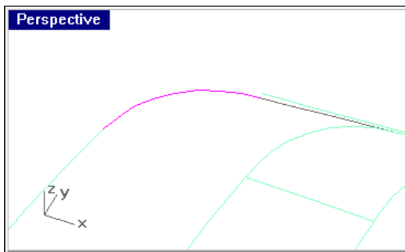
Designer's transom blended to the projected swim step side curve.
